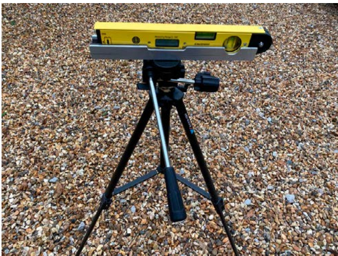
Fig. 3. Electronic clinometer (with 0.1-degree accuracy) in its 0.0^\circ closed position.
